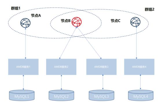
As shown in the above figure, NodeB belongs to multiple groups. The AMDB server and MySQL which are corresponded by the same node in different groups are separate. For distinguishing the same node in different groups, the nodes of A, B, and C are respectively represented with Group1\_A (NodeA in Group1, same as below), Group1\_B, Group2\_B, and Group2\_C.
