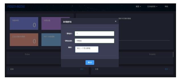
Once it is set up, users can access the front-end by typing IP and its port configured by nginx through web browser. Browser without group initialization will lead to new group configuration page, where the group ID, group name and group description are needed.
